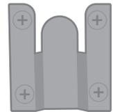
Finish the assembly of the left front panel with the left side panel by locking loops.
