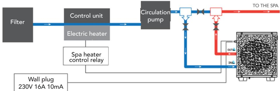
Note: Install your heat pump at the outlet of the filtration pump so that the flow sensor works. The flow sensor is used to ensure safe water flow. If it is not working, the heat pump will not start up.
