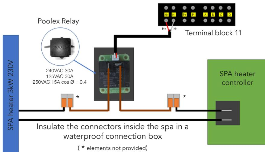
The SPA heater SPAWER driver system consists of a power relay (230V50Hz / 30A) which plugs into the heater phase wire (between the SPA heater controller output and the heater itself).
